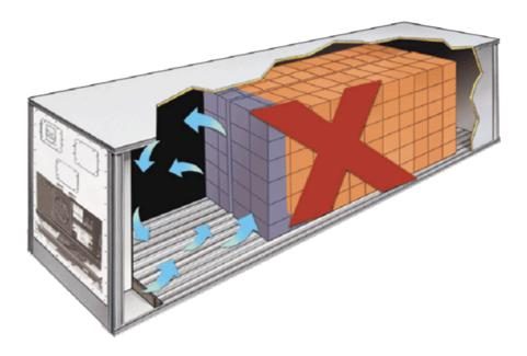
Load placed IN the front OF the container. Result: Air IS NOT forced through the interior OF the load
