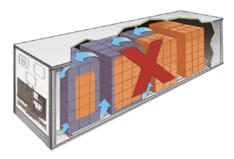
Load placed IN the rear OF the container. Result: Short cycling
