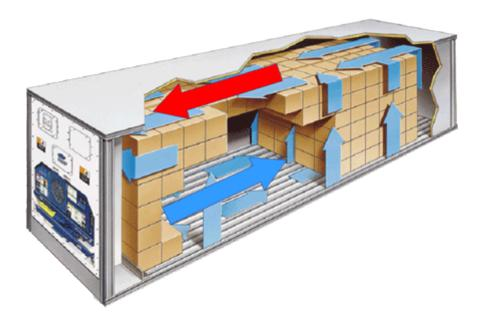
Excessive SPACE BETWEEN load. Result: Airflow doesn't extend the FULL LENGTH OF the container
